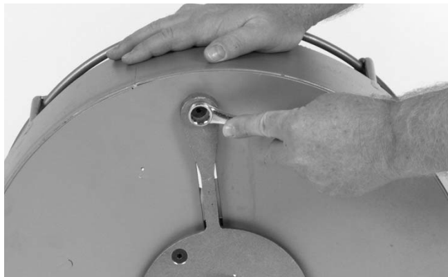
Figure 12 – Removing Pigtail Anchoring Bolt
