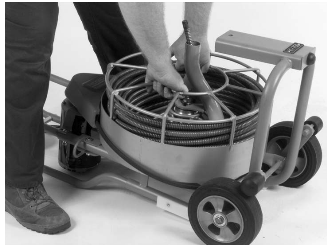
Figure 11 – Lift Drum From Mounting Position
