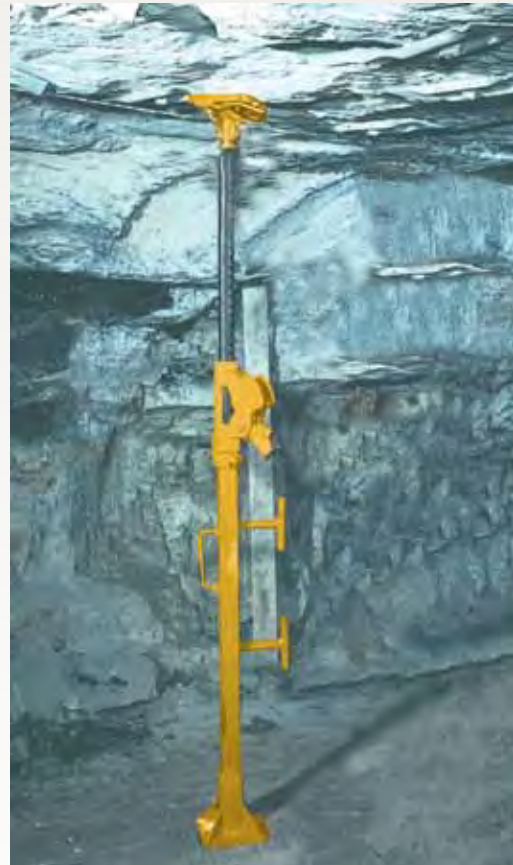
S Type Head 36 square inches in support area.
