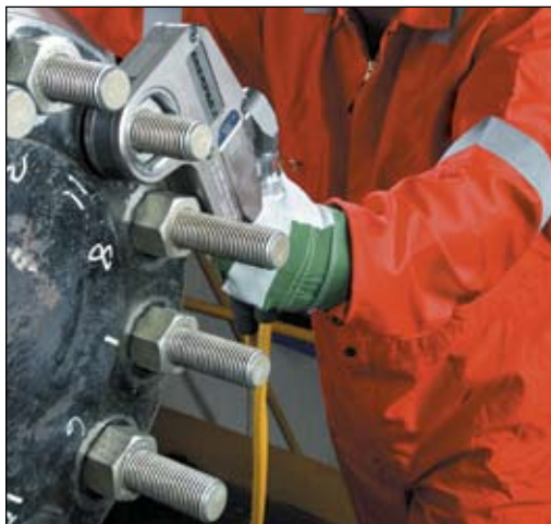
◀ Most hydraulic torque wrenches can be powered by the Enerpac ZA4T-Series torque wrench pump.
