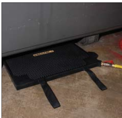
◀ An Enerpac LB-6 lifting bag preparing to lift a CNC machining center.
